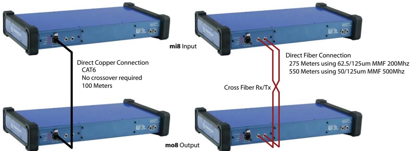
Optionally, Fiber and Copper may both be connected for redundancy.
