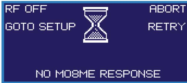
The Tweak will go to the **Communication Time Out Screen** if the **mo8me** is not powered up or if the address is incorrect. This screen could also appear if a communications error occurs while Tweak is in use (i.e. User steps outside of the wireless range). If the Network is up and the address is correct, this screen will be skipped.
