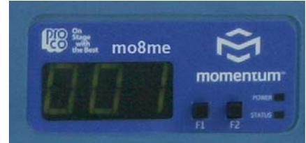
It is best practice to keep the input unit's IP address sequential with its channel. In other words, Chn 001-008 would be Adr 001 and Chn 009-016 would be Adr 002 and so on.
